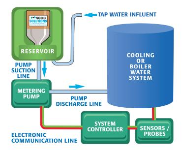
Existing system monitors and testing procedures are used to measure SOLID SOLUTIONS product concentrations in the systems. Operating parameters such as molybdate concentrations, pH levels, conductivity, and microbiological counts will still be periodically evaluated by a designated Jamestown Service Engineer to maintain continuous and consistent levels of performance.
